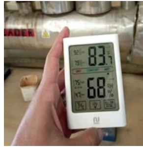
Gambar 9. Pengecekan kelembapan ruangan boiler .
