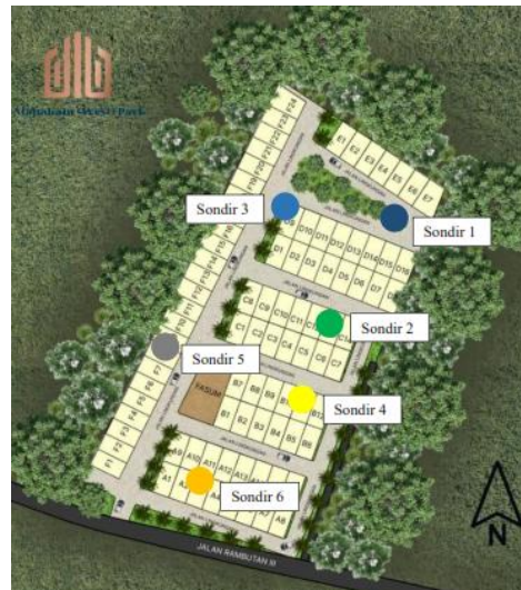
Figure 2. Cone Penetration Test (CPT) locations (Source: Project documentation, Mahakam West Park Residential Development, Pekanbaru)
